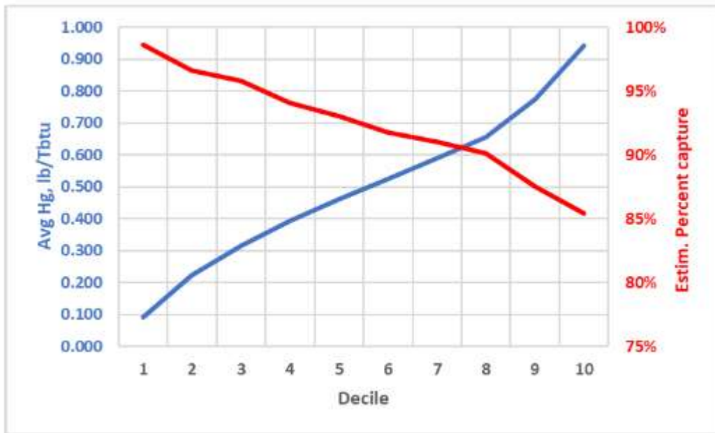
Figure 13. Average Hg concentration and estimated percent capture by decile for not-low-rank virgin coal 54
