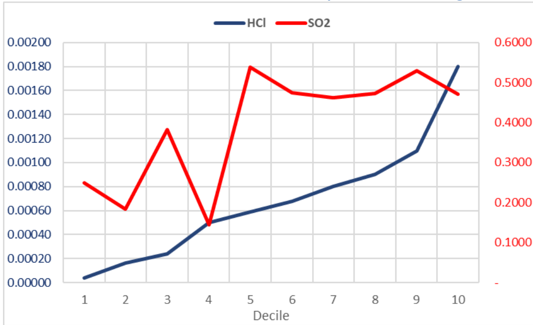
Figure 35. Median HCl and SO 2 emissions rates based upon decile according to HCl emissions
