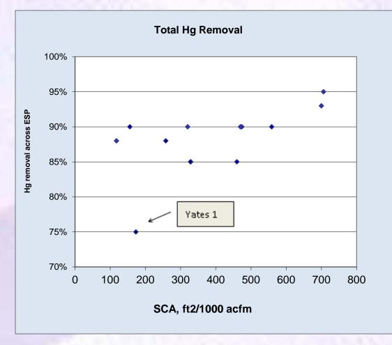
Hg capture doesn't seem impacted by ESP size without SO3 conditioning.
