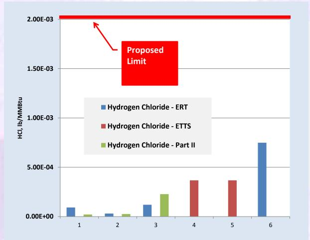
Acid gas emissions from TX lignite were well below limit, no doubt from high concentration of alkaline fly ash.
